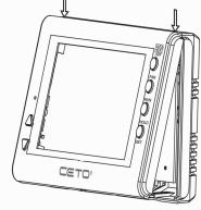
Step 2: Hang the two hooks of the front part at 30° right to the snaps.
