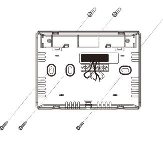
For horizontal mount put one screw left and one screw right.
